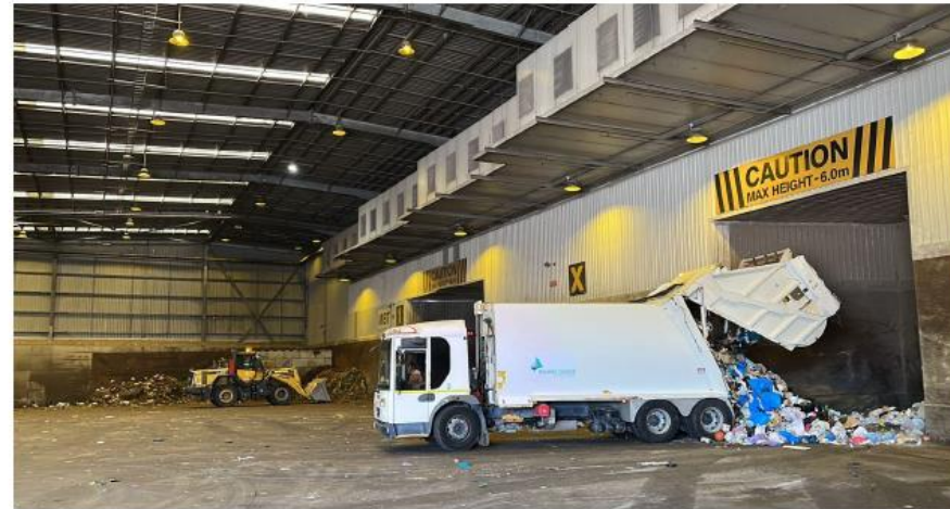
Banksmeadow (NSW) receival pad, compactor opening and high velocity fans
