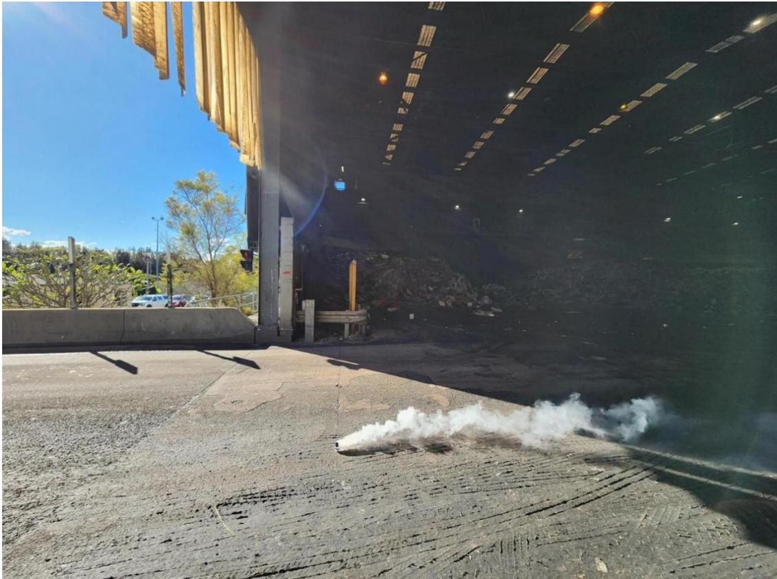
**Photo 2.4** – A view of the truck entrance plastic strips during smoke testing on 5 July 2023
