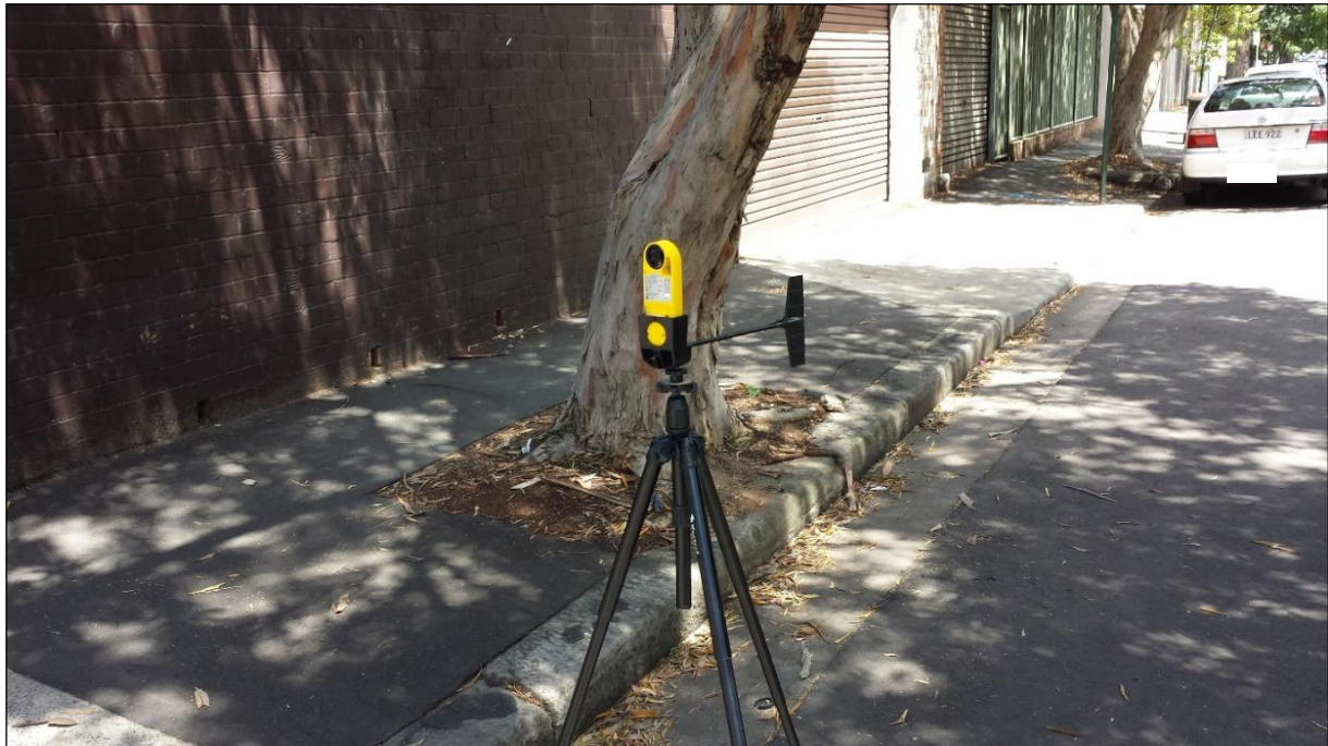
Photo 7.1 - Illustrated setup of the Kestrel Anemometer apparatus in operation (Source: TOU)
