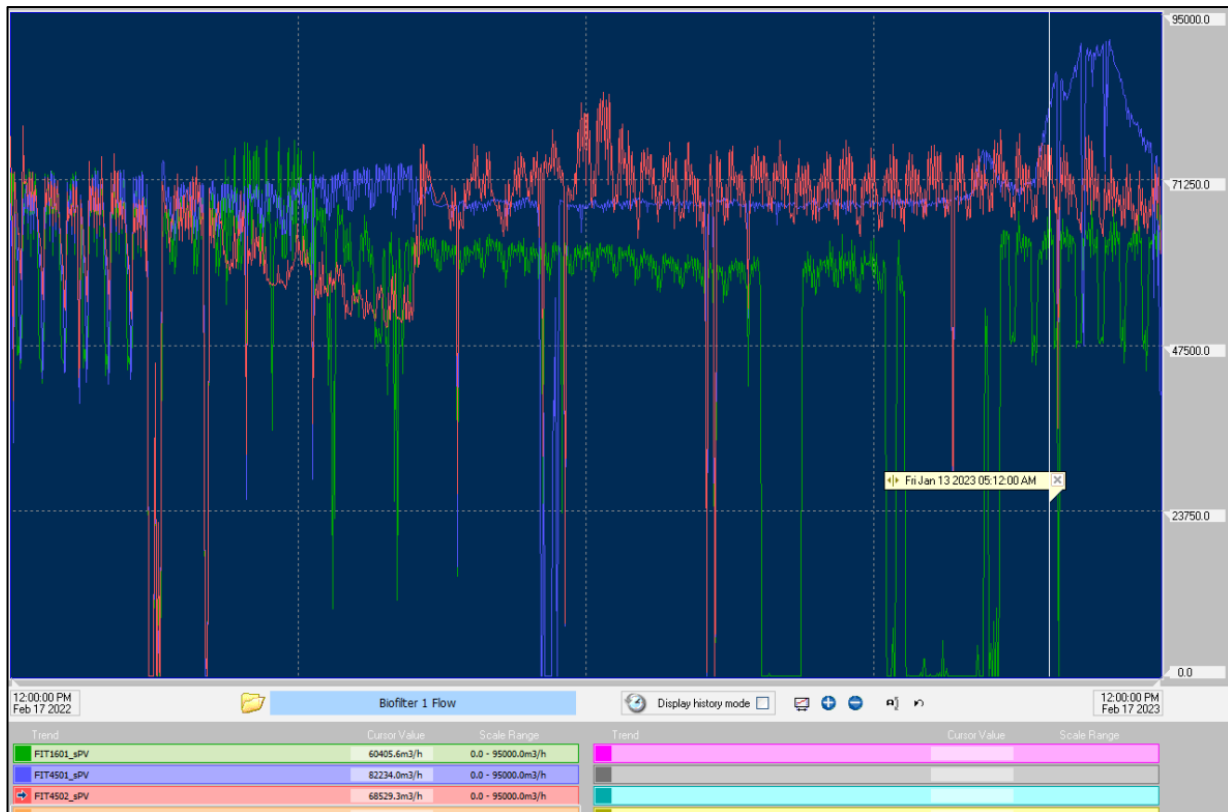
Figure 9.7 - An example of the biofilter airflow monitoring records retrieved from the SCADA system for Odour Control System 1 and Odour Control System 2 at the MBT Facility
