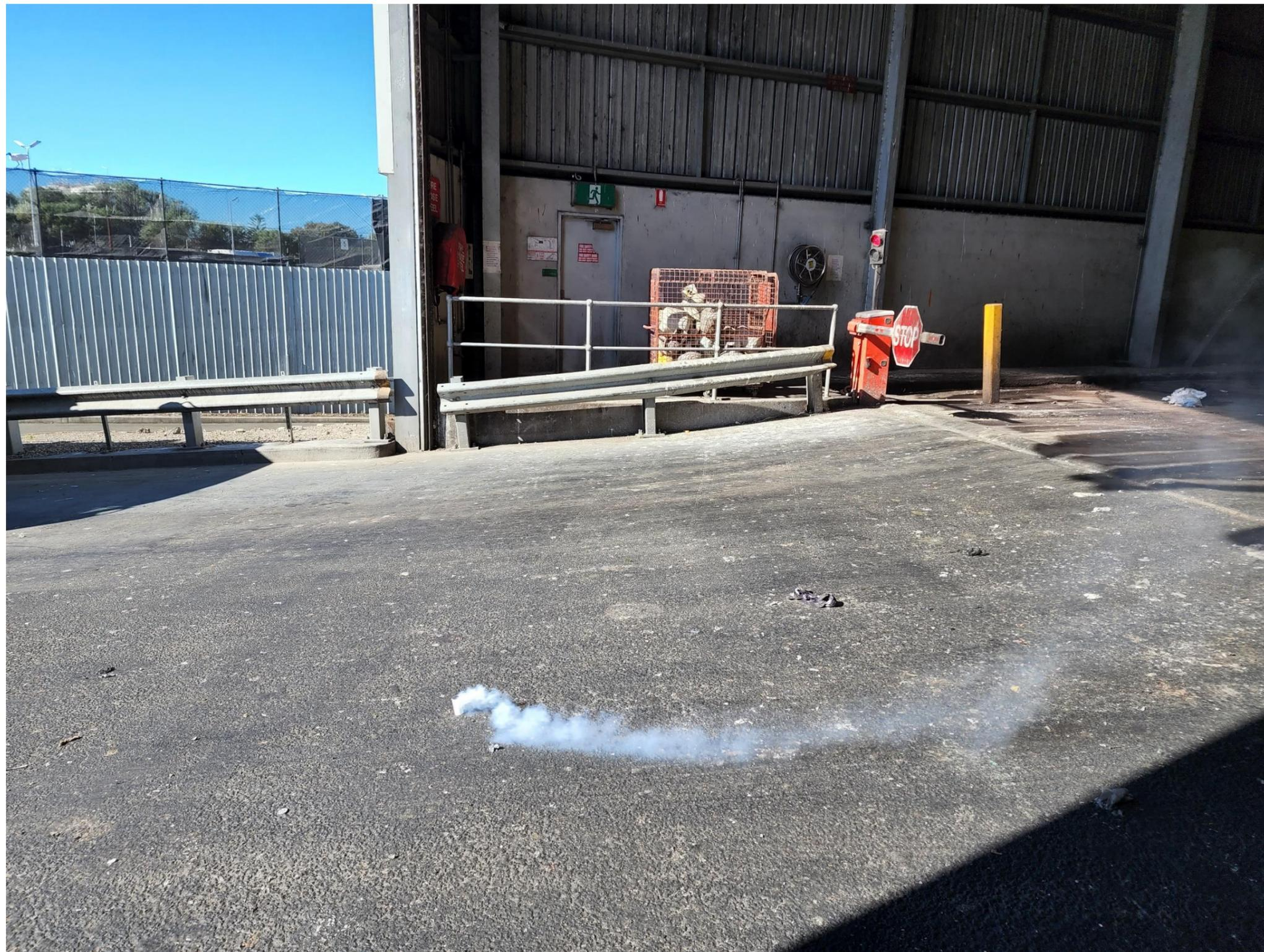
**Photo 2** – Smoke testing at the truck entry point of the BTT Facility building enclosure on 1 June 2022
