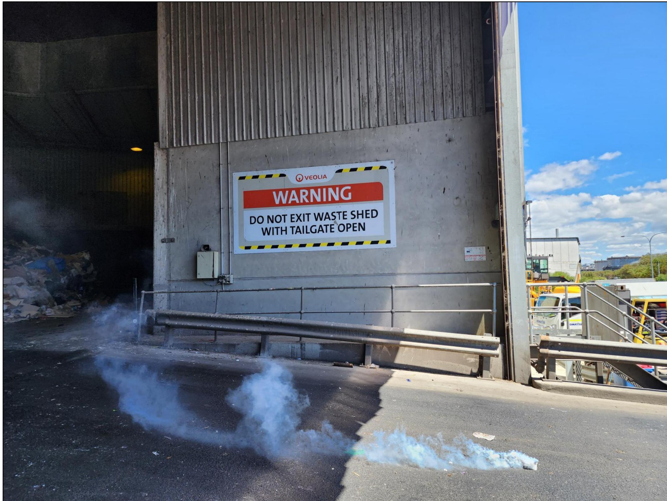
**Photo 2** – Smoke testing at the truck entry point of the BTT Facility building enclosure on 21 December 2022
