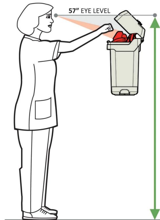
Identify the location and height for the container placement. Place the wall mount flush against the wall and level it from side to side and back to front. An ideal standing installation height for a fixed sharps disposal container is 1.35m. This height will comfortably accommodate 95% of all adult female workers.
