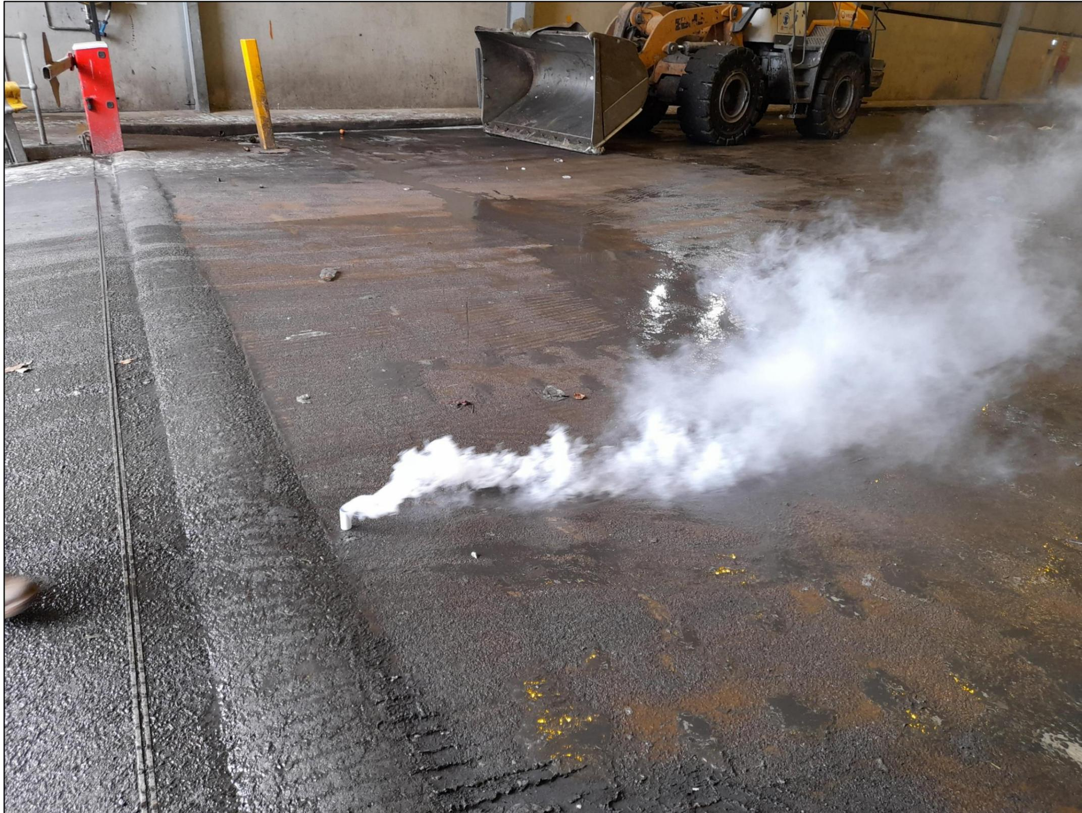
**Photo 2** – Smoke testing at the truck entry point of the BTT Facility building enclosure on 25 November 2021 at 0953 hrs
