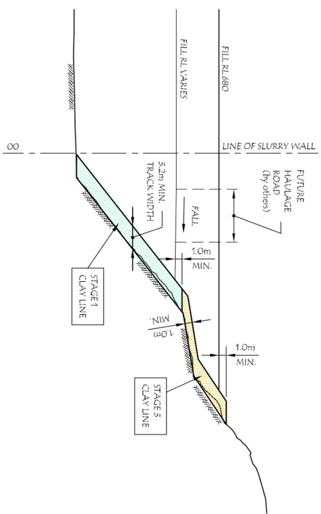
TYPICAL SECTION THROUGH STAGE 1 & 3 LINER
