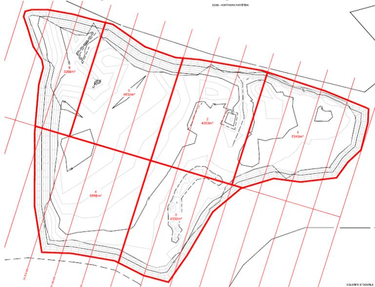
2. The contractor shall rip up the existing material from the floor to a depth of 1,200mm. This material will be removed and stockpiled on another segment to enable a base level survey to be undertaken.
