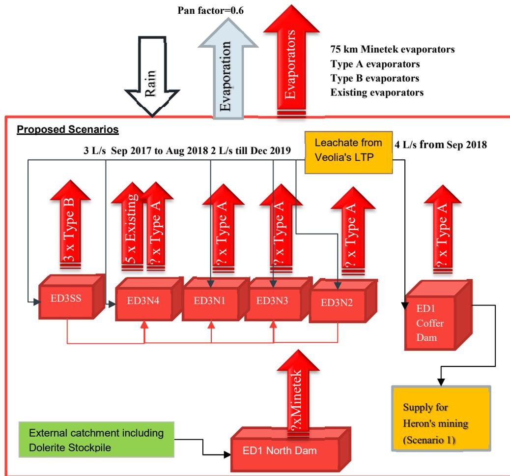
Figure 4.1 Schematic representation of modelled dams in GOLDSIM
