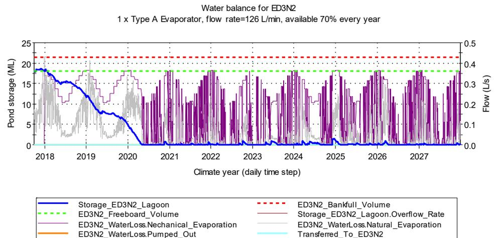
Figure 7.31 Simulated result for ED3N2 in the average climate sequence
