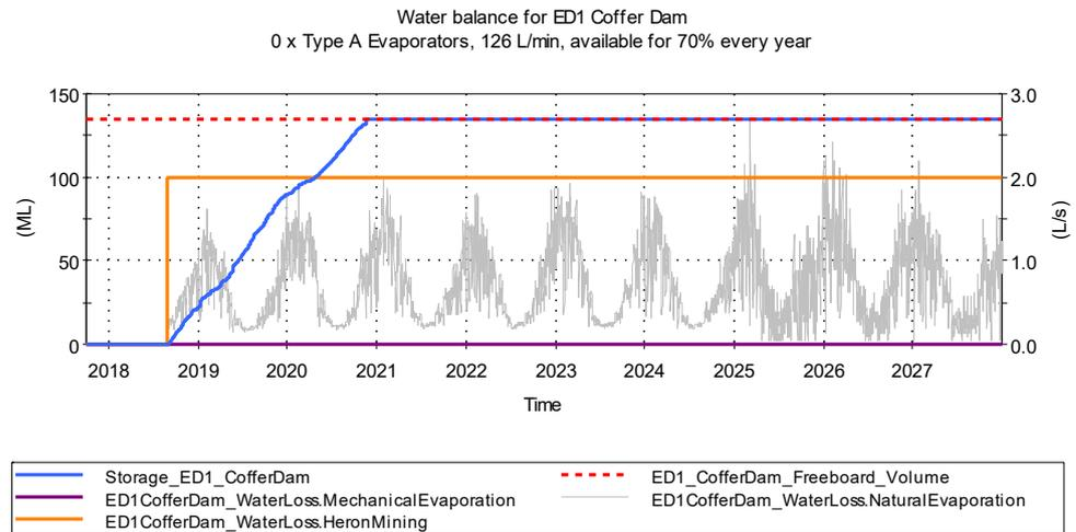
Figure 7.3 Simulated daily time series for the 150 ML ED1 Cofferdam Scenario 1C
