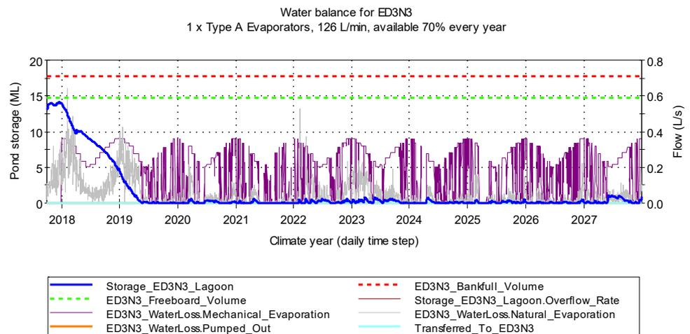
Figure 7.27 Simulated result for ED3N3 in the driest climate sequence
