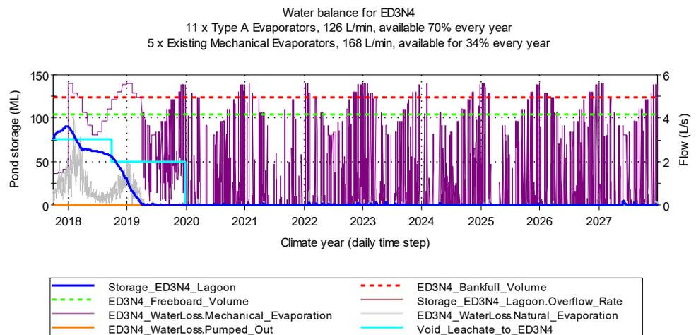
Figure 7.28 Simulated result for ED3N4 in the driest climate sequence
