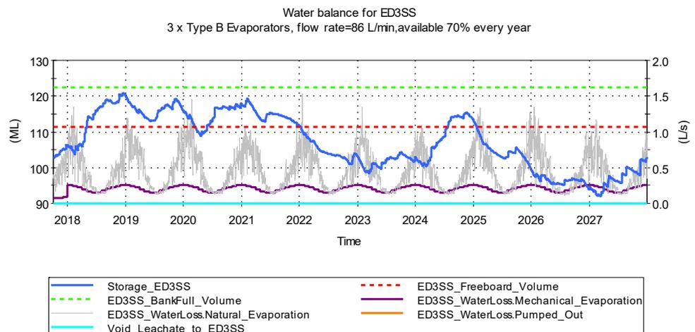
Figure 7.19 Simulated result for ED3SS in the wettest climate sequence
