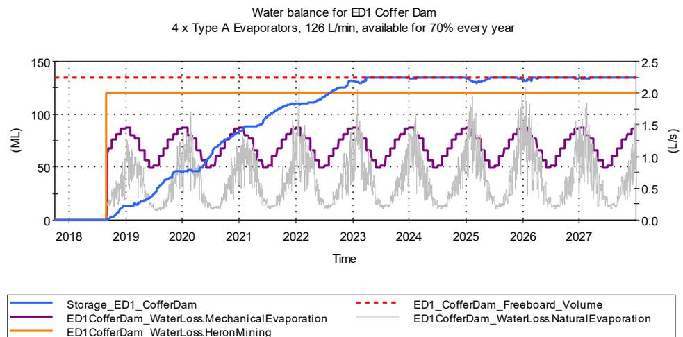
Figure 7.4 Simulated daily time series for the 150 ML ED1 Cofferdam Scenario 1D
