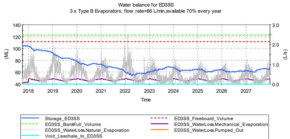
Figure 7.24 Simulated result for ED3SS in the driest climate sequence
