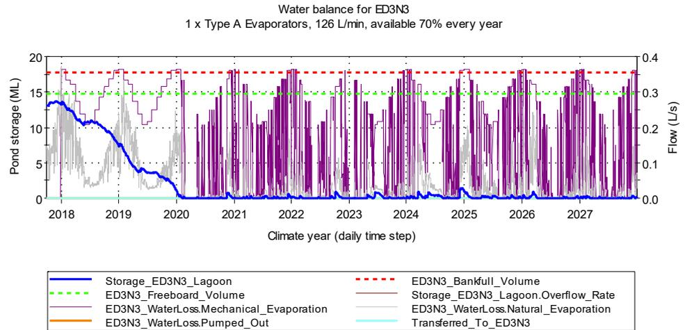
Figure 7.32 Simulated result for ED3N3 in the average climate sequence
