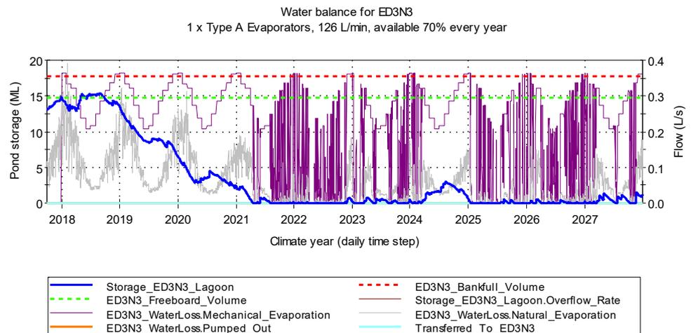
Figure 7.22 Simulated result for ED3N3 in the wettest climate sequence
