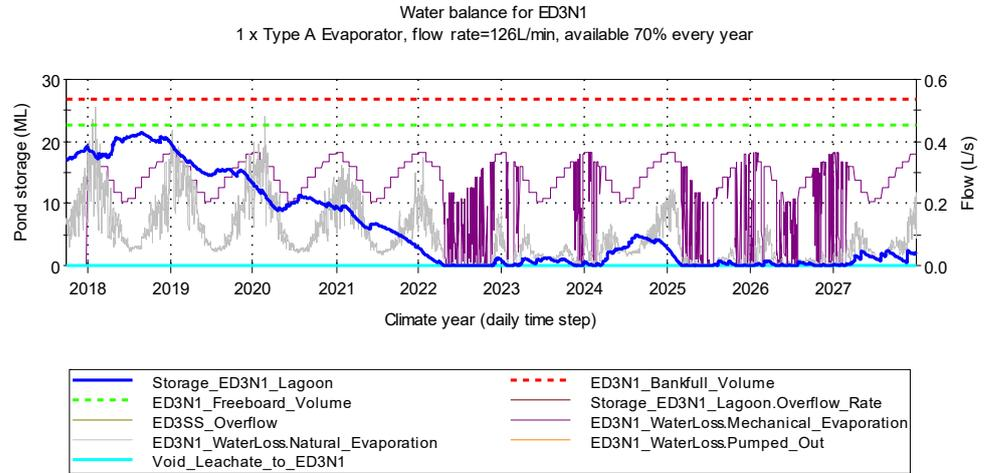
Figure 7.20 Simulated result for ED3N1 in the wettest climate sequence
