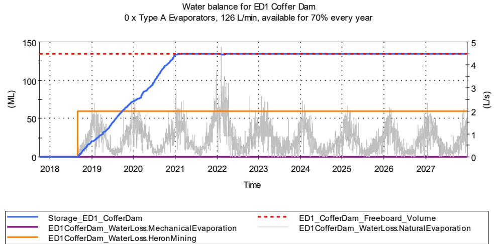
Figure 7.2 Simulated daily time series for the 150 ML ED1 Cofferdam Scenario 1B
