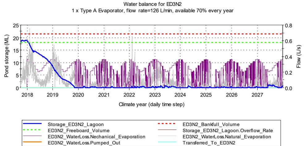
Figure 7.26 Simulated result for ED3N2 in the driest climate sequence
