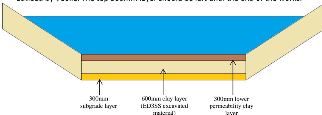
9. Insitu density tests and permeability tests will be collected at various depths over the liner. The final surface will be surveyed to verify thickness of the 900mm layer and the 300mm layer.
