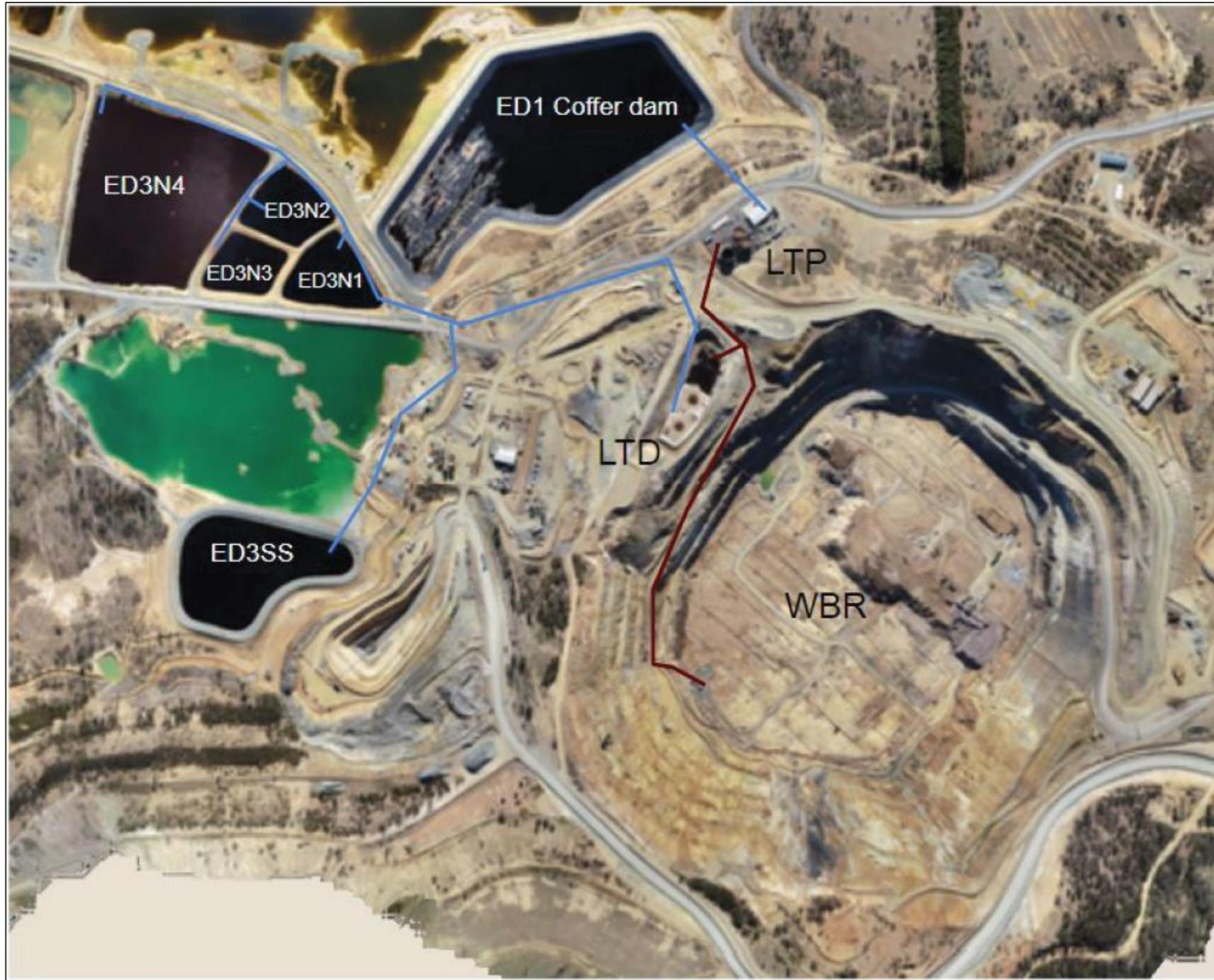
Figure 2.10 - Concept layout of the LMS for the Bioreactor at the Woodlawn Facility (Source: WIP 2020)
