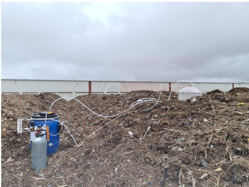
**Photo 4.1** - An example of IFH sampling on a solid surface (Maturation Pad Stockpile at the MBT Facility) as occurred on 24 March 2022
