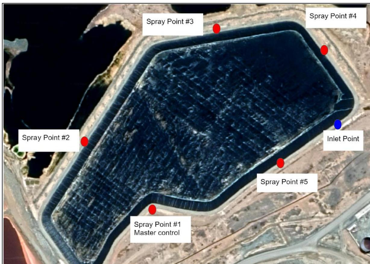
**Figure 2.6** – ED1 Cofferd Dam: Proposed Evaporation Spray System (**Source:** WIP 2020)
