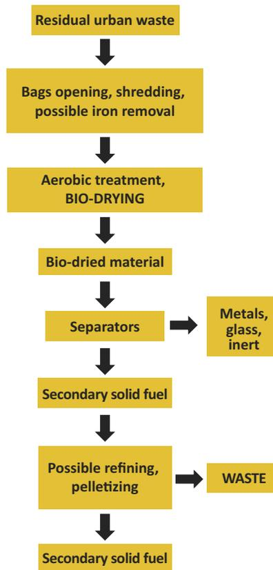
**Figure 5.2** - Diagram of an MBT with biostabilisation process
