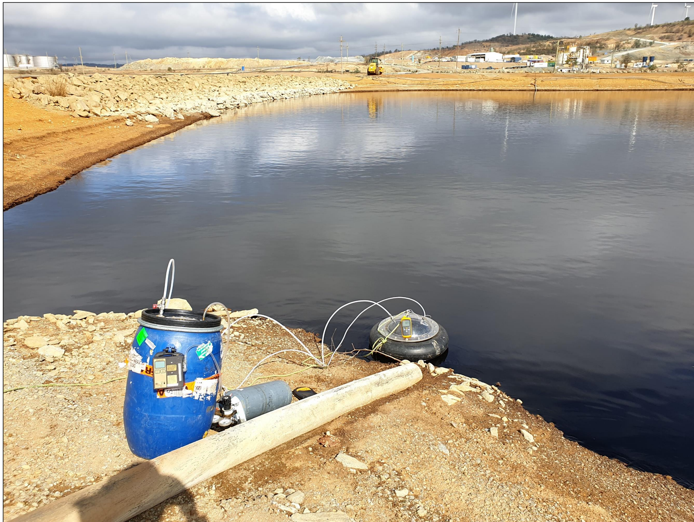
Photo 4.2 – An example of IFH sampling on a liquid surface (ED3N-2) as occurred on 17 February 2020
