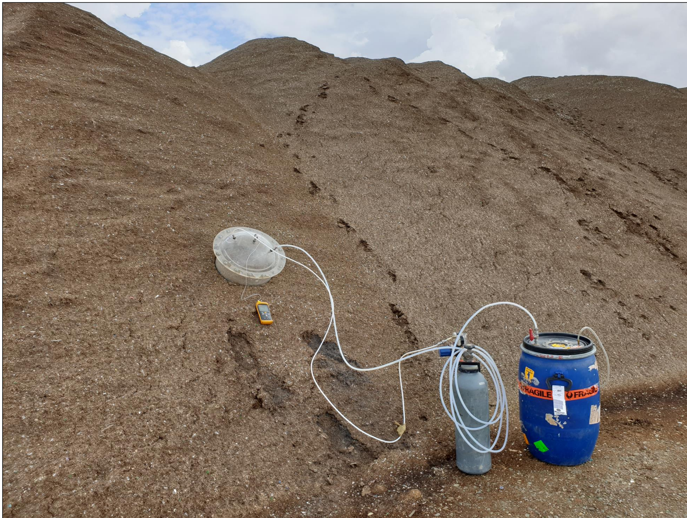
Photo 4.1 – An example of IFH sampling on a solid surface at the MBT Facility as occurred on 18 February 2020
