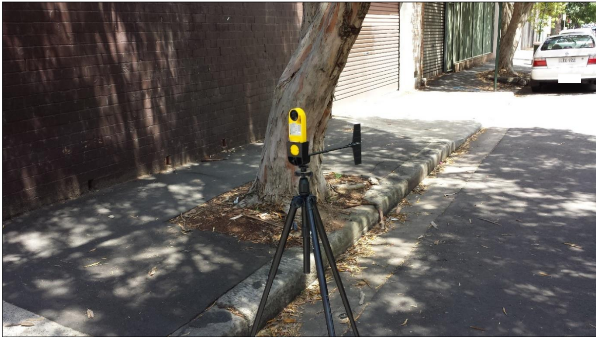
Photo 7.1 - Illustrated setup of the Kestrel Anemometer apparatus in operation (Source: The Odour Unit Pty Ltd)
